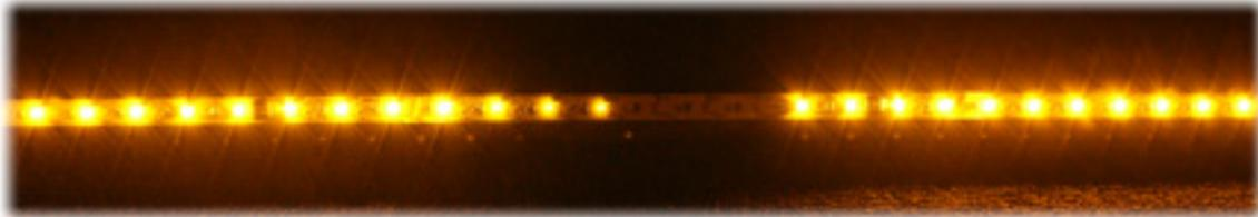
**Strips of LEDs on the LCI-2 Bus, showing different brightness levels per LED**
