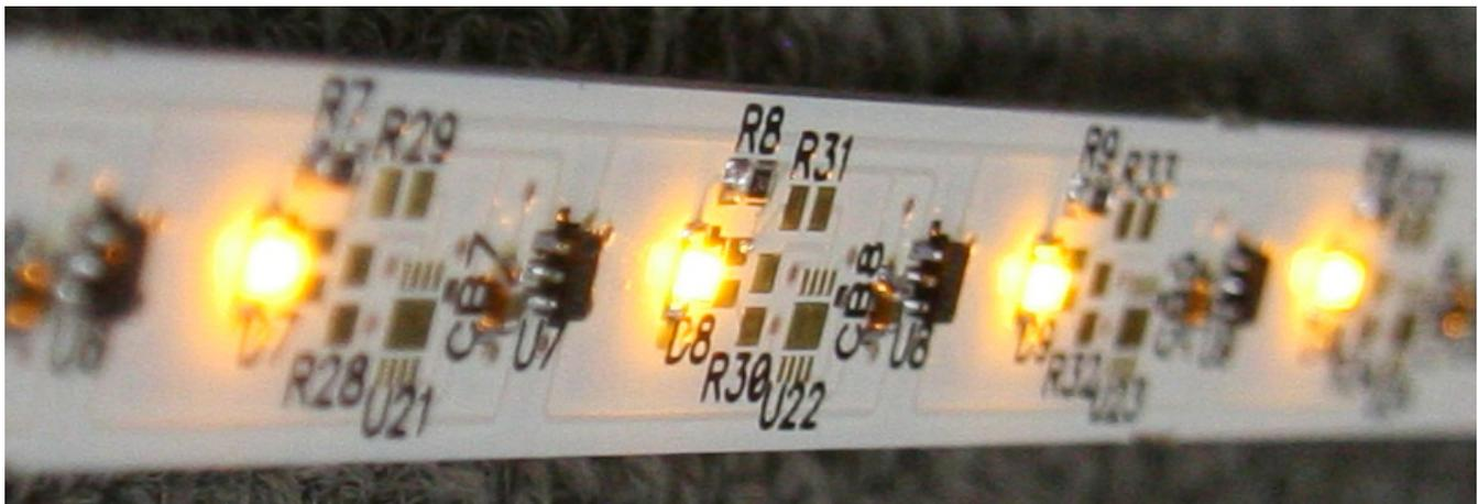
**Close up of individual LEDs and their associated LCI Node Chips.**
