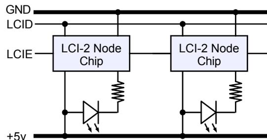
The LCID and LCIE signals originate at the LCI Bus Master Controller. This controller sends out a serial stream of commands on the LCI Bus, which is then picked up by all the individual Node chips. This allows a controller to completely control one entire LCI Bus full of lights.
