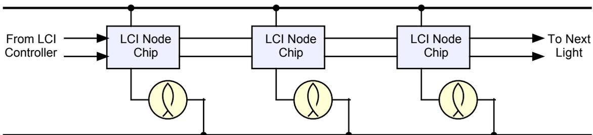
**Figure 2 - The LCI Node Chip Typical Wiring**
